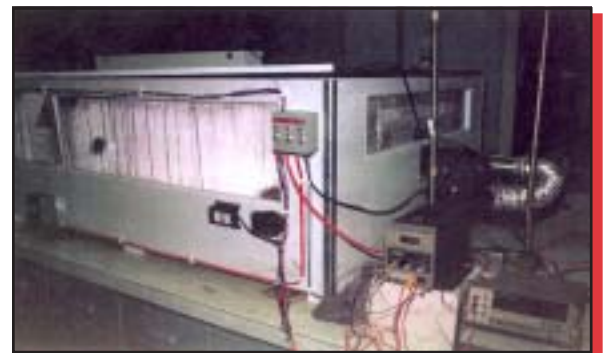
Corrosion Chamber Simulates Prolonged Exposure To The Harshes Environment
