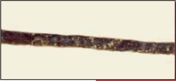
Close-up (25X) of scribe(scratch) PROTECTED by the Final Coat Module
