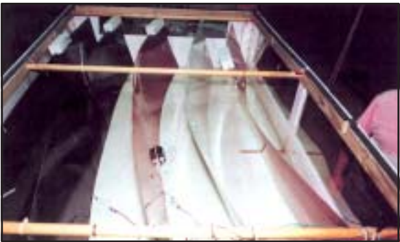
Protected Sheet Metal Test Panels & Unprotected Control Panels Are Scribed And Exposed To 500 Hours of Humidity @ 95° F
